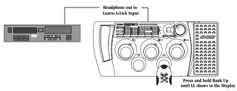
. Press the number 1 footswitch as you start your tape or CD player. The display will show  $\tau \Gamma$  indicating that it recording. It will record 16 seconds of incoming material. The Parameter Edit LEDs will light one at a time as our record time is used.
